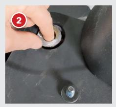
• Position the 2 x 'top hats' over the rear mounting holes so that they fill the holes in the rubber floor mat
