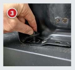
• Remove 2 x front seat nuts (16mm socket spanner for front 2 bolts)
