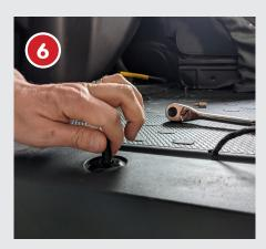
• Remove the 2 front bolts sticking up through the floor (T30 torx bit)
