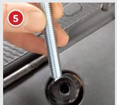
• Use the enclosed 50mm bolts and washers for the front fixing points (these replace the original threaded rods that you have already removed)
