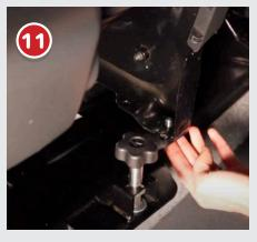
In the back right corner, use the enclosed 10mm bolt and a washer (feed them in from below) and fix with a washer and nut
