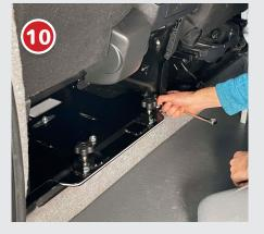
• Use the nuts and washers to attach the two front and the rear left corner of the seat
