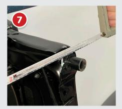
• Cut off the 2 x 'top hats' under rear of seat frame. (Use a hack saw between the main seat frame and 'washer', then prise off with an old screwdriver). Note: the removed pieces will get used again so don't lose them!
