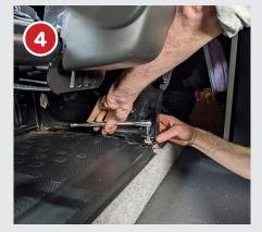
• Remove 2 x rear fixing bolts (11mm socket)
