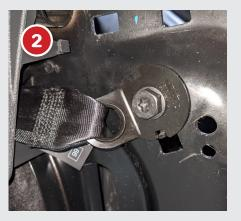
• Detach seat belt from the side of the seat (17mm socket spanner)
