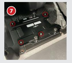
• Remove the nuts and washers from the upward pointing bolts on your swivel
