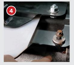
• Use the original 2 x thick washers and original bolts to fix the rear of the swivel
