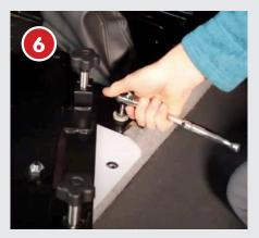
• When attaching swivel to the van floor, take care to work your way around all 4 fixings gradually tightening each in turn (so that you avoid twisting the swivel plates)
