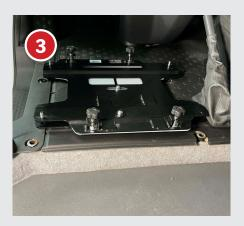
• Position swivel in place (reinforcing bars to the rear) so that the rear fixing holes are aligned on top of your 'top hats'
