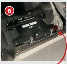
• Remove the loose upward pointing bolt from the back right corner of the swivel
