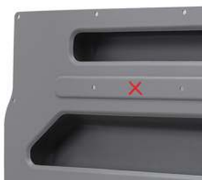
Press firmly on the ridge (X) with one hand while inserting popper with the other
